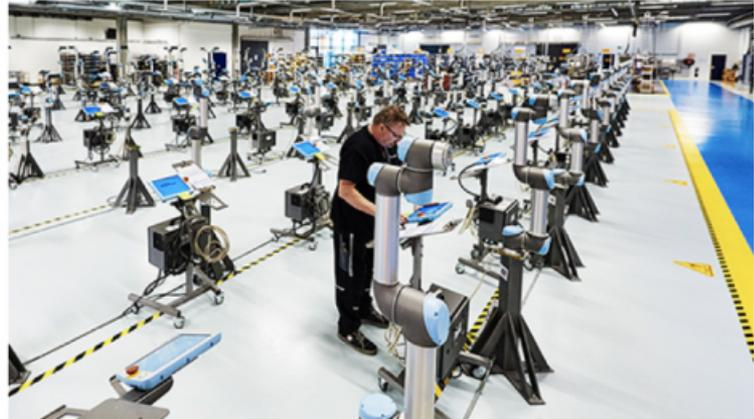
A collaborative robot (“co-bot”) is a robot designed to share a workspace with humans and may have direct physical interaction with humans. (Collaborative robot can be a subset within the broader industrial robot definition.)
